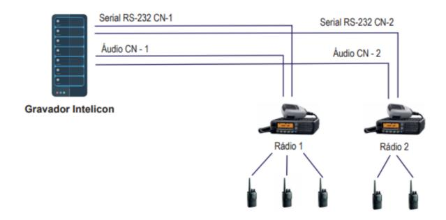
Radio audio recording is accomplished by connecting the radio loudspeaker output to a channel in the Intelicon Call Recorder radio interface board. Recording works independently of RS-232 serial port communication. The RS-232 connection is used to provide radio ID only.
